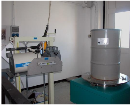
MGAS (Mobile Gamma Assay System), based on ISOCS
