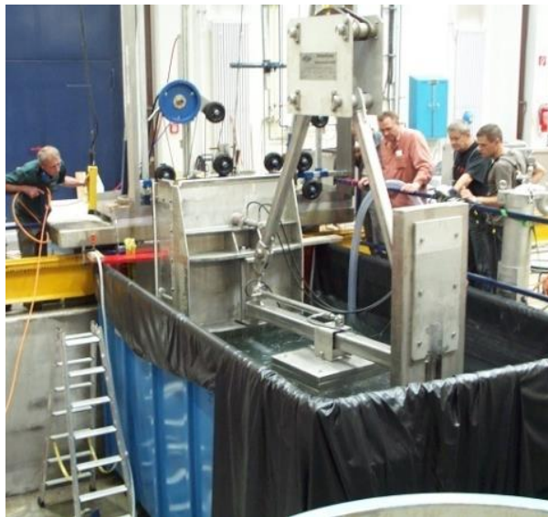
Wire saw cutting of stainless steel brackets
