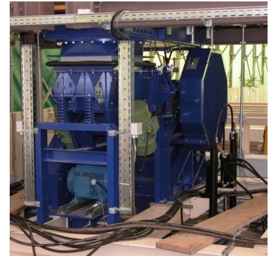
Concrete crusher for waste processing and packaging
