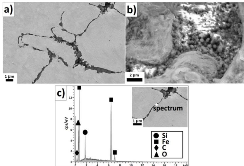
Fig.2: a) cross-section view of coated Fe particles (bright phase) after 17 hours of synthesis, with visible coating layer (dark phase) between the particles, b) SEM image of Fe particles (surface view) with  $\text{SiO}_2$  nanoparticles, rarely spherical shape, c) EDX analysis of coating formed on the interface of two particle.
