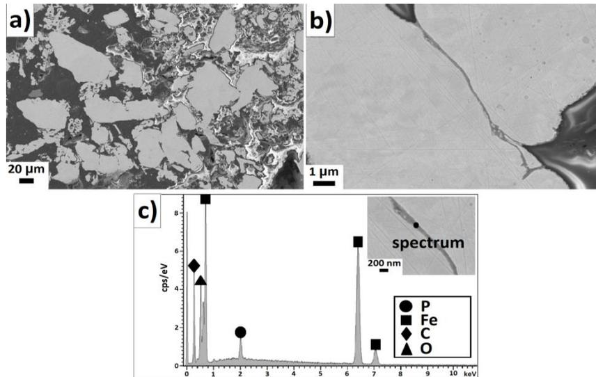
Fig.1: *a) cross section view of coated Fe particles (bright phase) embedded in resin (dark phase), b) detailed look on a interface between two particles with visible coating between them, c) EDX analysis of formed coating proved the presence of phosphorus.*
