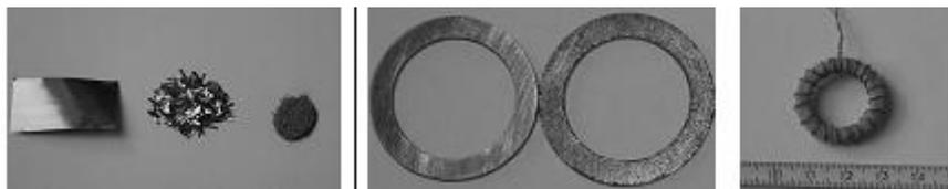
Fig.1: Sample preparation process (thin foil, cut foil, powder, rings and rings prepared as a coil with turns for ac and dc measurements).
