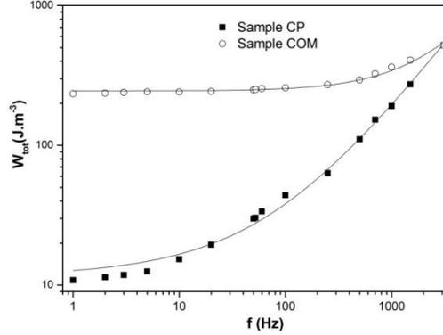
Fig.3: Total losses  $W_{tot}$  of both samples as a function of frequency. The symbols denote experimental results and lines are fits according to Eq. (2) and Eq. (3).
