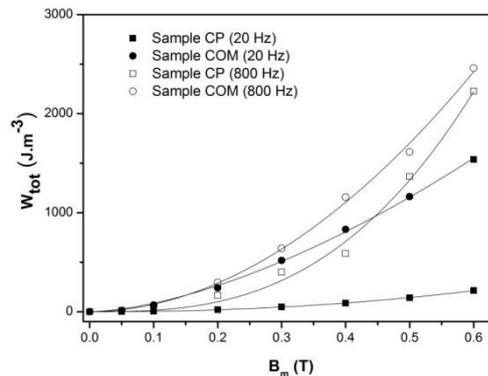
Fig.4: Total losses  $W_{tot}$  both samples as a function of maximum induction to 1.2 T. The symbols denote experimental results and lines are fits according to Eq. (4).
