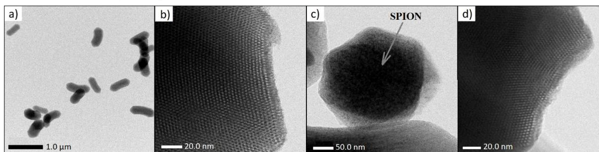
*Fig. 1: a) mesoporous silica MCM-41; b) a blank mesoporous silica MCM-41 higher resolution; c) mesoporous silica containing iron oxide nanoparticles MCM-41@Fe<sub>2</sub>O<sub>3</sub>; d) mesoporous silica with drug MCM-41@naproxen.*
