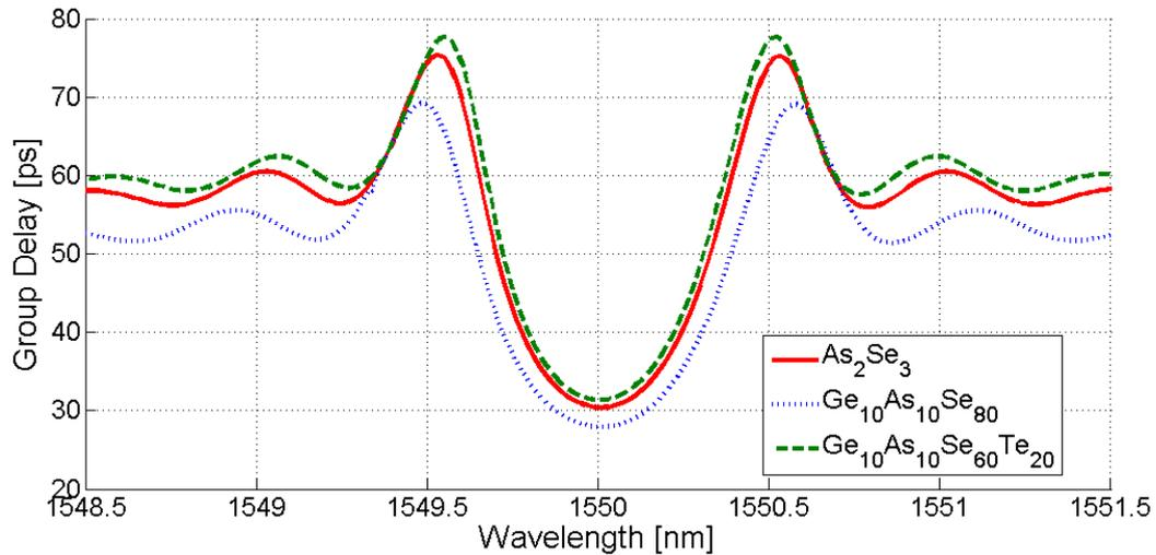
Fig.2: Wavelength dependency of group delay for the gratings with neglecting the nonlinear effects.
