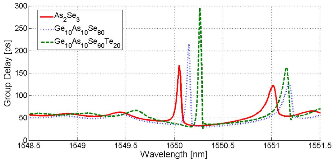
Fig.3: Wavelength dependency of group delay for the gratings at intensity  $250 \text{ MW/cm}^2$ .
