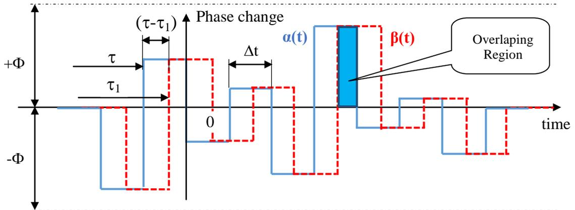
Fig. 2: Arbitrary („white-noise“ like) phase modulation functions  $\alpha(t)$ ,  $\beta(t)$  delayed in time by  $(\tau - \tau_1)$ .
