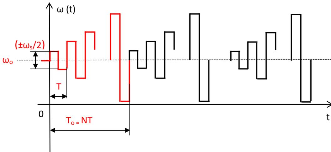
Fig. 4: Periodical stepwise frequency modulation function of the laser source, one step period is  $T$  and the total period  $T_0$ ,  $T_0 = NT$
