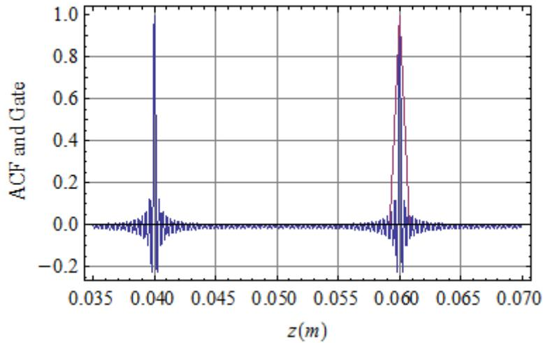
Fig. 5: First two peaks of the laser source periodic autocorrelation function with the “gate” at the second peak position
