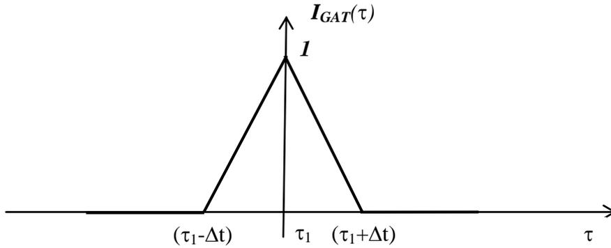
Fig. 3: The shape of the “extraction gate” obtained by the synchronization of the phase modulation functions of the testing signal and the signal in reference arm.
