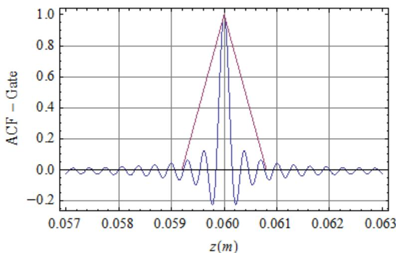
Fig. 6: Detail position of the “gate” with respect to the second peak of the synthesized autocorrelation function
