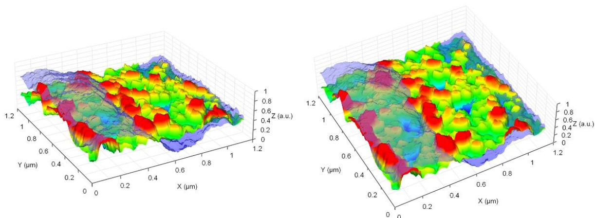
Fig.2: *3D imagination of height profile representing grain structure (red-green) and phase profile representing domain structure (blue). Two different views. The interaction between grain structure and magnetic domain is well observable. (colour online)*
