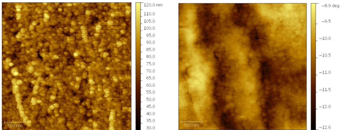
Fig.1: *MFM scan, (3x3) $\mu\text{m}$ , height profile (left panel) and phase profile (right panel). Surface and magnetic measurements were made in two different scans using a very accurate navigation of the measuring tip. (colour online)*
