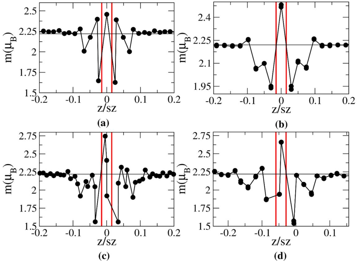
Fig.3: Variation of local magnetic moments of Fe atoms at GBs (a)  $\Sigma 5(210)$ , (b)  $\Sigma 5(310)$ , (c)  $\Sigma 17(410)$ , (d)  $\Sigma 13(510)$ . The positions of atoms are presented with respect to the supercell size ( $sz$ ). Experimental bulk magnetic moment value  $2.22 \mu_B$  is indicated by horizontal solid line and GB plane is positioned between two vertical lines. [3]
