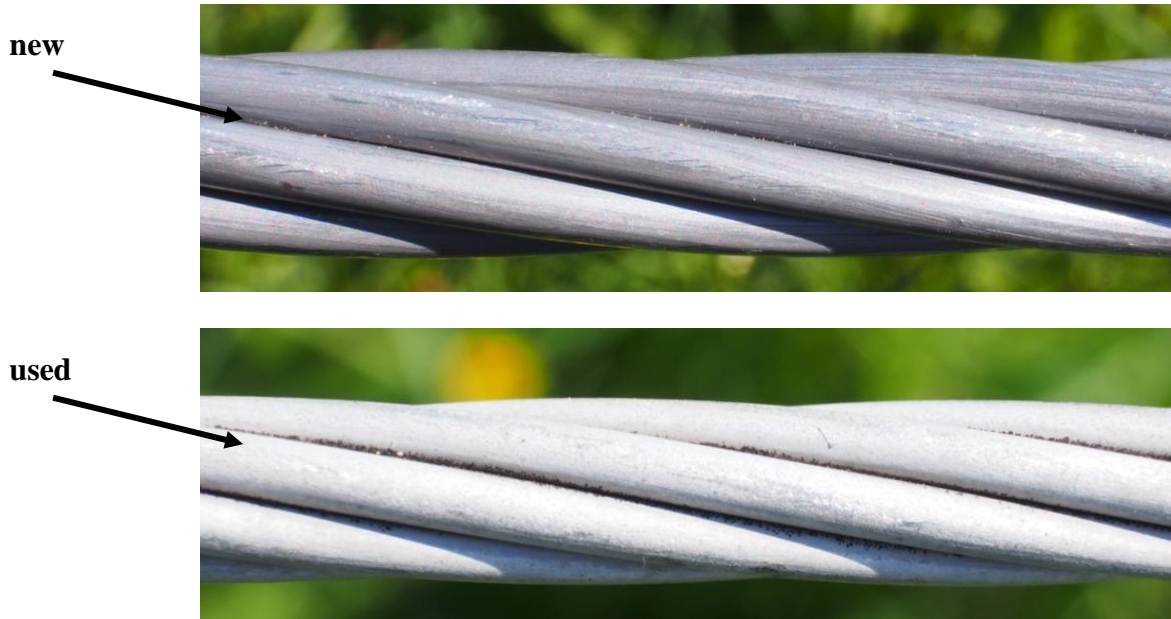
Fig. 3. Detail of the new and the used AlFe power line
