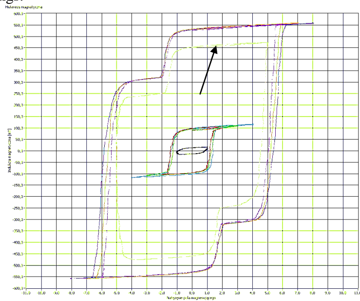
Fig. 2 B(H) loops measurement results, value of magnetizing field H \div 10\text{ A/m}
