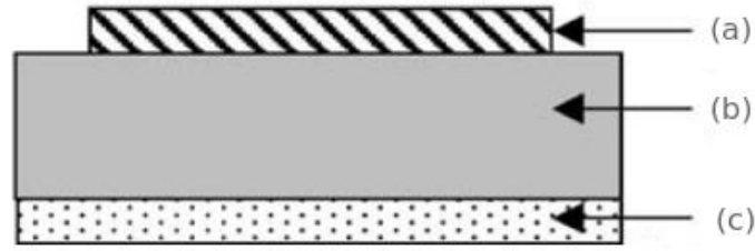
Fig. 1: Cross-sectional view of the investigated Schottky contact SI GaAs detector: (a) Ti/Pt/Au Schottky contact (b) bulk SI GaAs (c) Ni/AuGe/Au metal electrode
