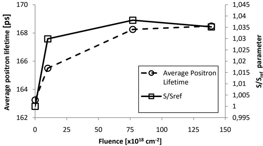
Fig. 1: Irradiation dependence of average positron lifetime and  $S/S_{ref}$  parameter of positron annihilation spectroscopy techniques
