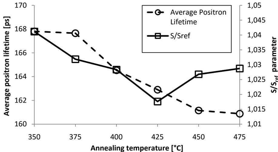
Fig. 2: Annealing temperature dependence of average positron lifetime and  $S/S_{ref}$  parameter of positron annihilation spectroscopy techniques
