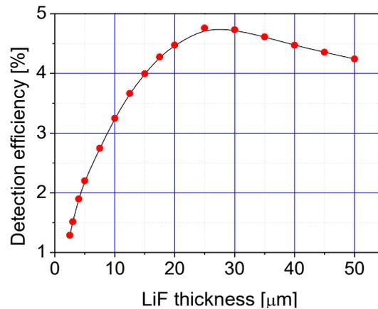
Fig.2: Detection efficiency of  ${}^6\text{LiF}$  layer as a function of its thickness.
