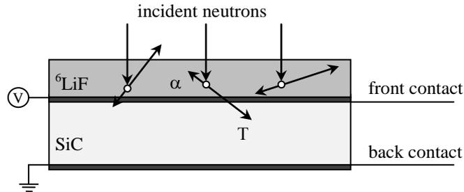
Fig.1: *Illustration of the thermal neutron detection principle.*
