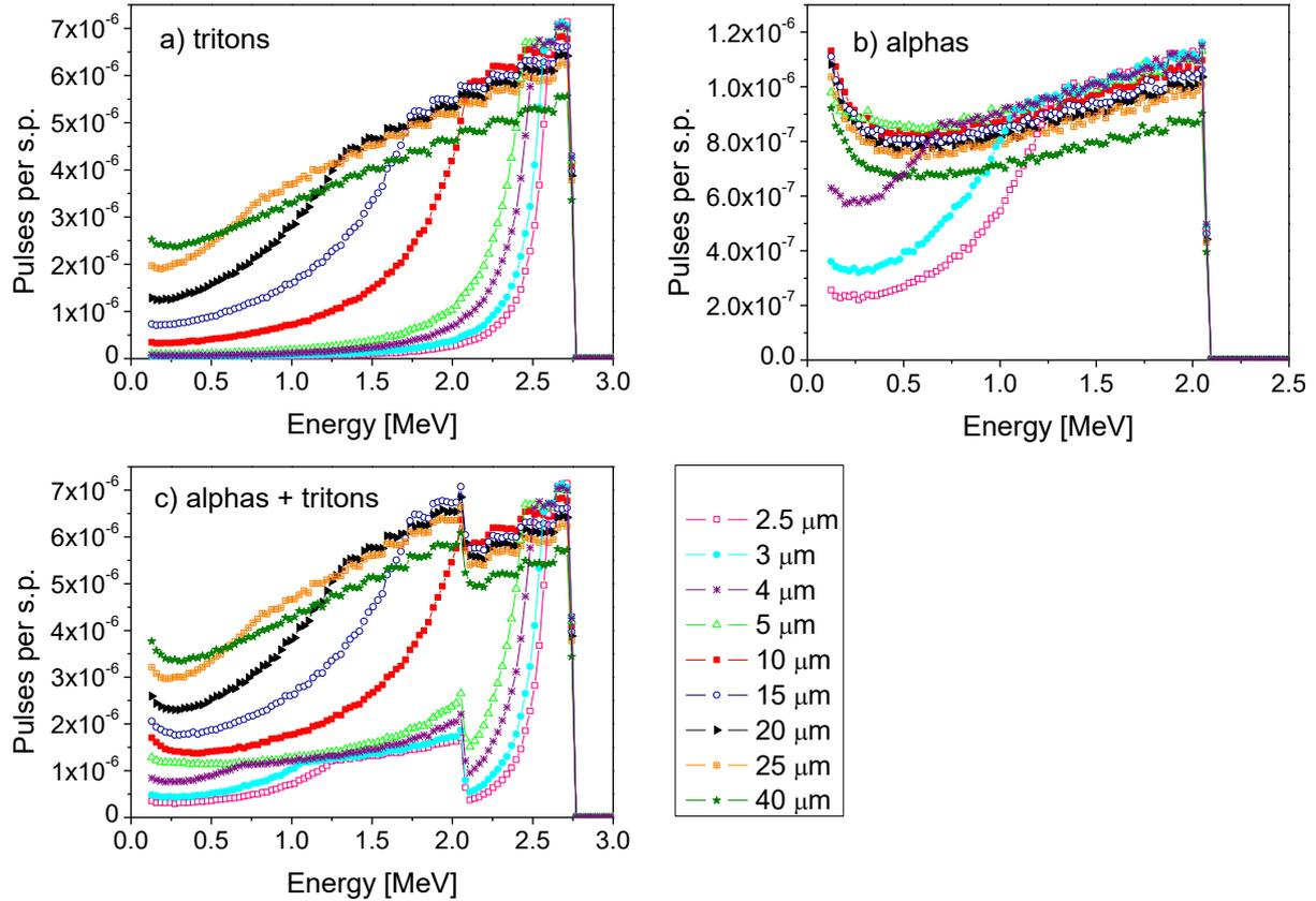
Fig.3: Contribution to the SiC detector response from tritons ( $f8:t$ ), a), and from alpha particles ( $f8:a$ ), b), and the total SiC detector response ( $f8:t + f8:a$ ), c), all of them plotted for different  ${}^6\text{LiF}$  layer thicknesses.
