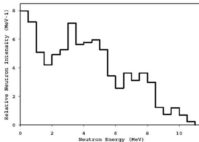
Fig.2:Pu-Be neutron source spectra.
