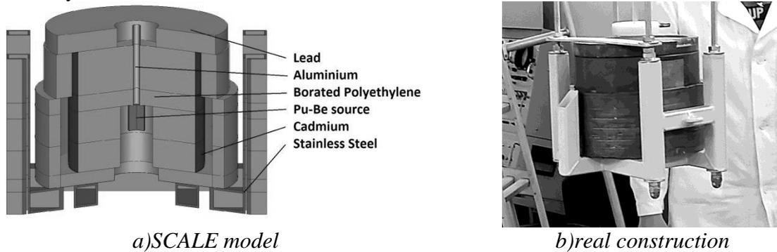
Fig.3: Transportation container geometry.
