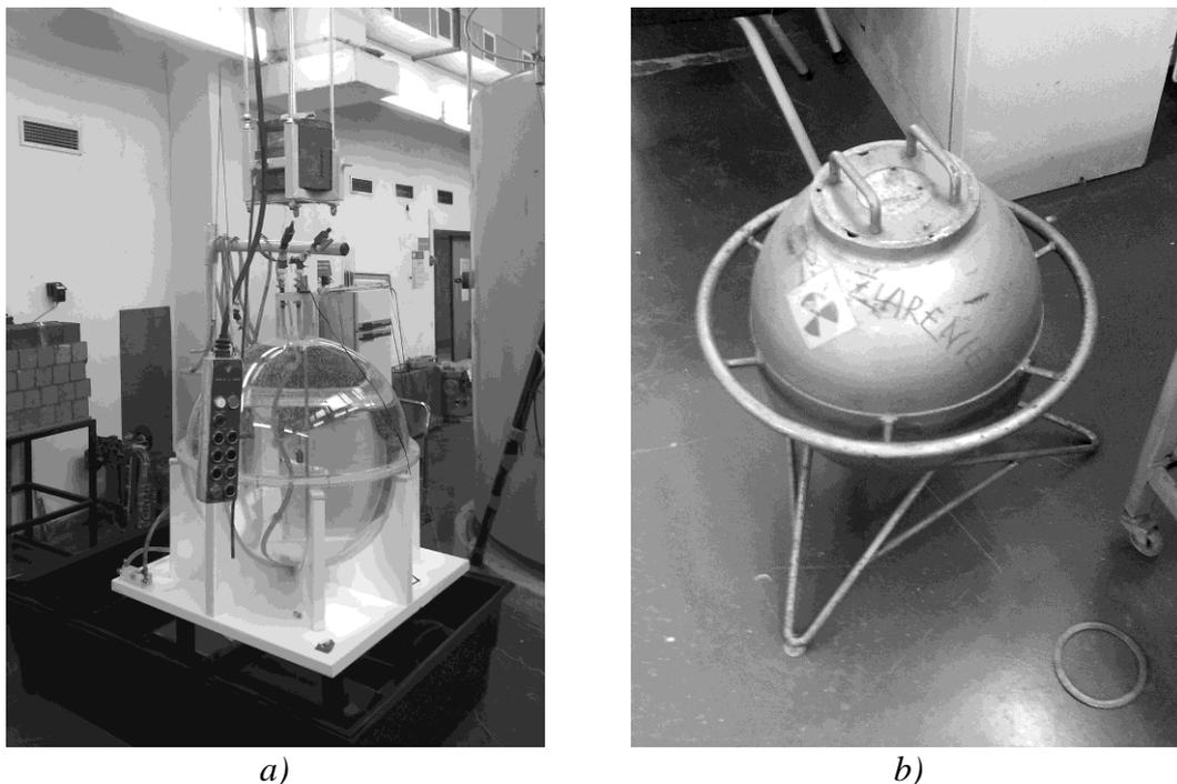
Fig.1: Manganese sulphate solution vessel and Pu-Be storage container.
