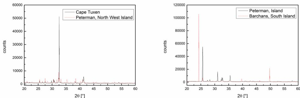
Fig. 4 X-ray diffraction patterns of gabbro (left) granodiorite (right) from different locations.
