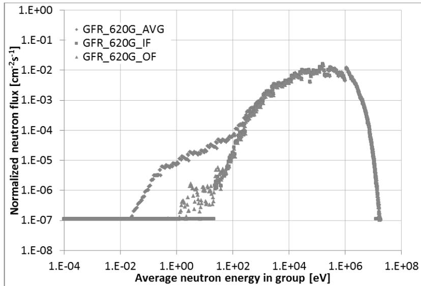
Fig.4: Comparison of neutron spectra at various positions in the GFR 2400 core
