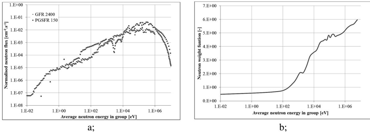
Fig.2:a - GFR 2400 and KALIMER 150 neutron spectra b- KALIMER 150 adjoint flux[14]
