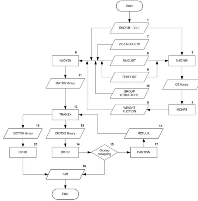
Fig.3: The cross section processing scheme
