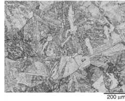
Fig.2.1: Microstructure of 15Kh2MFA steel [2].
