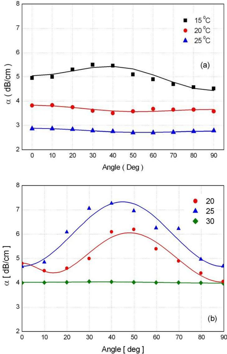
Fig.3: Anisotropy measurement of the acoustic wave attenuation ( $B= 200$  mT) for (a) MF MOGUL and (b) MF TECHNOL.
