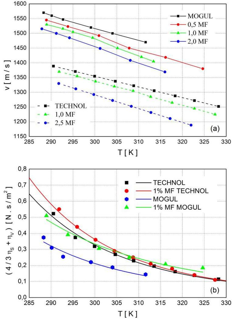
Fig.1: The velocity (a) and temperature dependences of term  $(4/3 \eta_S + \eta_V)$  (b) for various concentrations of magnetic nanoparticles in magnetic fluid based on MOGUL and TECHNOL.
