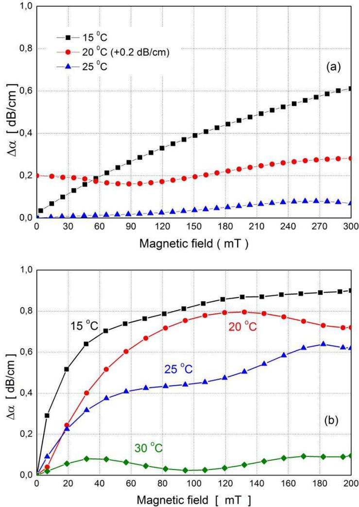
Fig.2: The dependence of acoustic attenuation changes on the external magnetic field for MF MOGUL (a) and MF TECHNOL (b) measured at various temperatures. Measurement at the temperature 20 °C in case (a) is shifted +0.2 dB/cm for better resolution.
