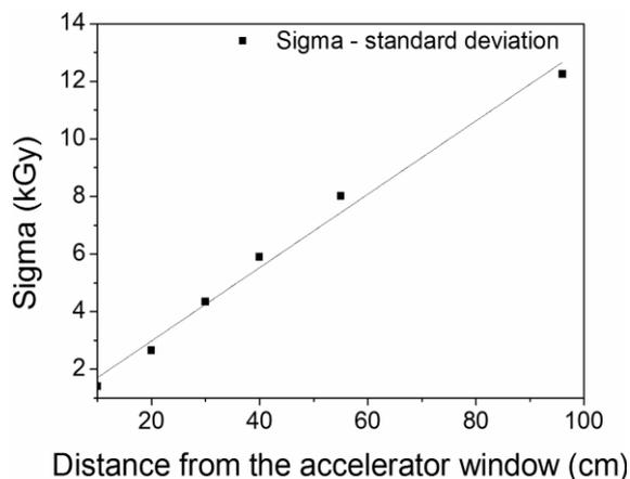
Fig. 3: Graph of the  $\sigma$  depending on the distance from the window of the accelerator.
