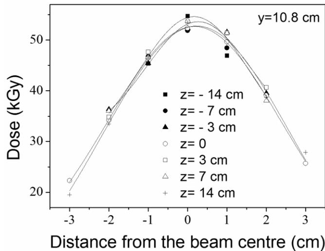
Fig.2: Graph of the measured dose depending on the position from the centre of the beam in direction perpendicular to beam scanning, at various positions along the scanning distance marked from the centre of the accelerator window (labelled z).
