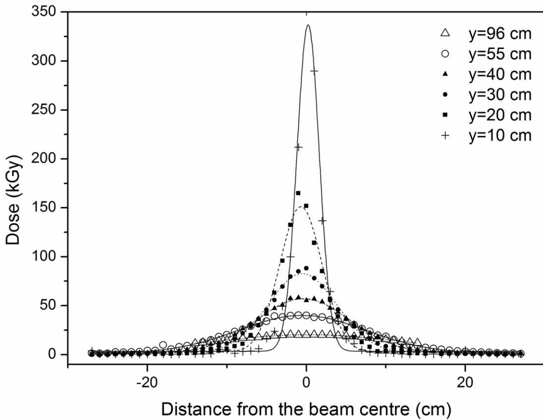
Fig.1: Graph of measured dose depending on the position from the centre of the beam in direction perpendicular to beam scanning, at various distances from the accelerator exit window (labelled y).
