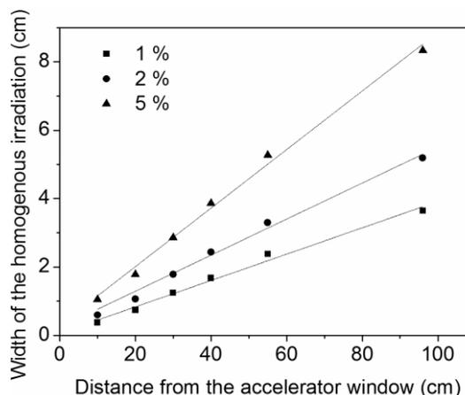
Fig.4: Dependence of object's maximum width on the distance from the window of accelerator. The object absorbed dose differs in 1 %, 2 % and 5 % of maximum dose.
