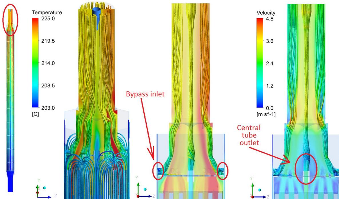
Fig.4: Bypass inlet to FA and central tube outlet coolant streamlines, coolant temperature and coolant velocity distribution in top part of FA (SST turbulence model )
