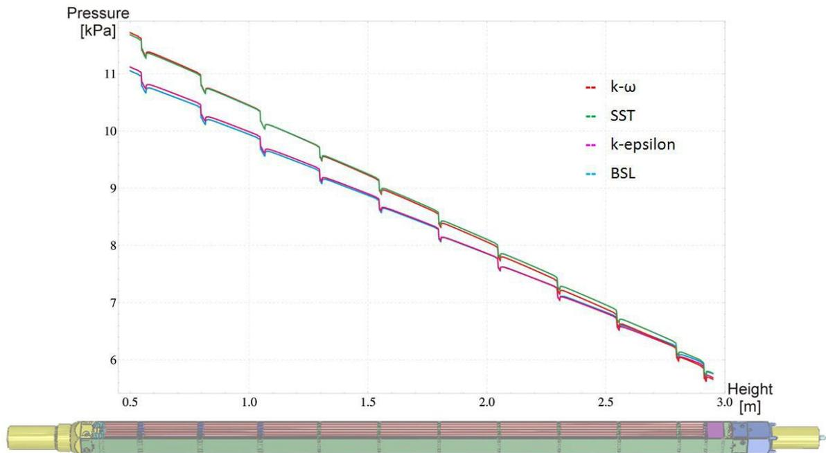
Fig.3: Dependence of pressure drop along the central tube height for used turbulent models
