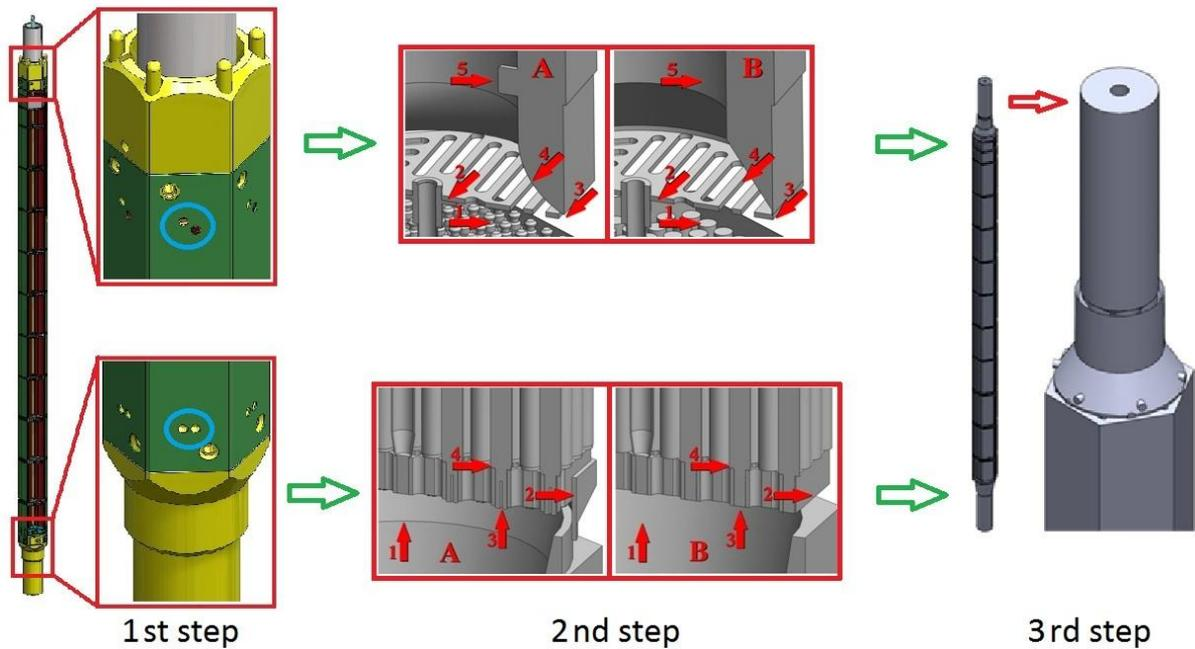
Fig.1: Detailed 3D CAD model of Fuel assembly (1st step), simplifications in particular areas (2nd step) and geometry model of coolant in fuel assembly (3rd step)
