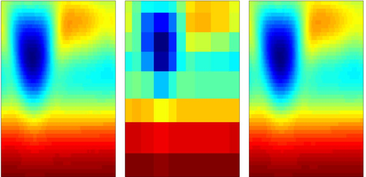
Fig.3: Exemplary results of described algorithm. Comparison of input data (left), points optimised for interpolation (centre) and interpolated results (right) present high efficiency of data reconstruction.
