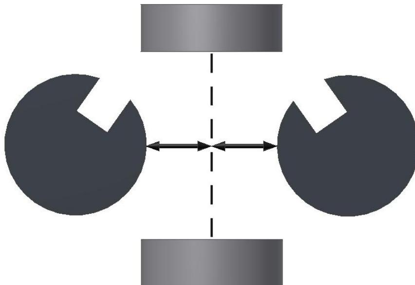
Fig.2: Visual explanation of results symmetry. Tested element is presented in two position. Second position is reflection of first with respect to the coils main axis.
