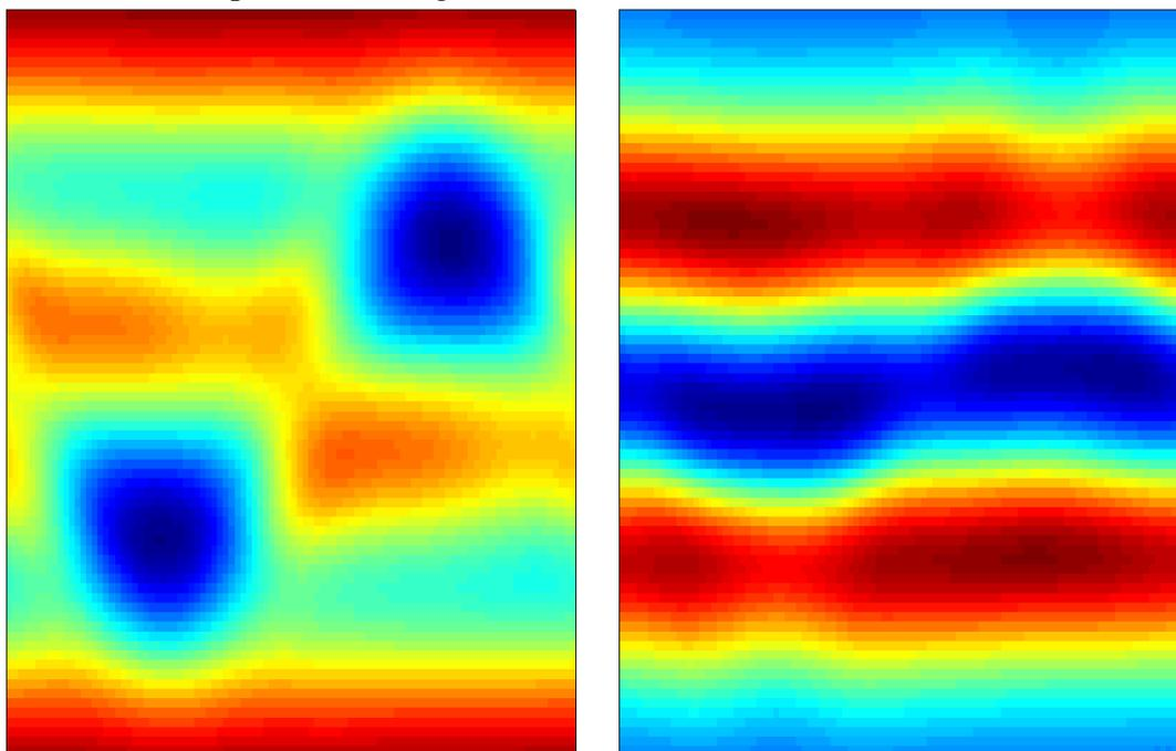
Fig.1: Exemplary results from eddy current tomography setup. Amplitude data (right) and phase data (left) are both presented in linear movement function (y axis) and rotation (x axis)
