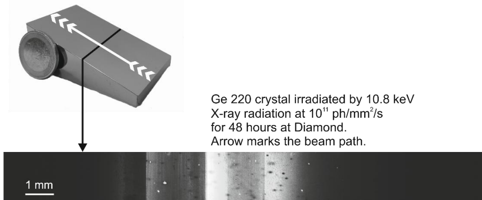
Mapping of surface damage using imaging ellipsometry (parameters to cancel reflection from pure Ge surface, \lambda=549 nm, P=52.6^\circ , A=29.9^\circ , C=45^\circ , a=60^\circ )
