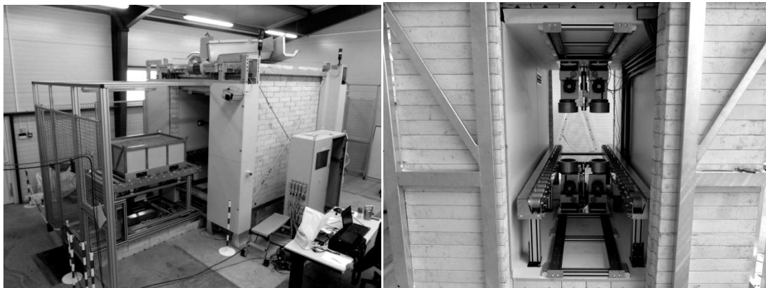
Fig.2. Radioactive waste free release measurement facility (MetroRWM experiment), general view and inner space with 4 HPGe detectors
