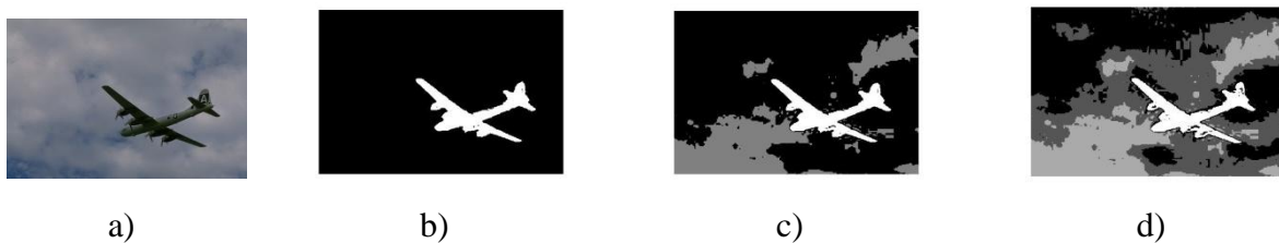
Fig.1: An image segmented by k-means algorithm. Figure a) original image, b), c) and d) original image segmented into 2, 3 and 4 clusters respectively.
