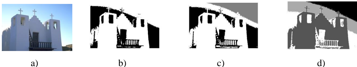
Fig.2: An image segmented by k-means algorithm. Figure a) original image, b), c) and d) original image segmented into 2, 3 and 4 clusters respectively.
