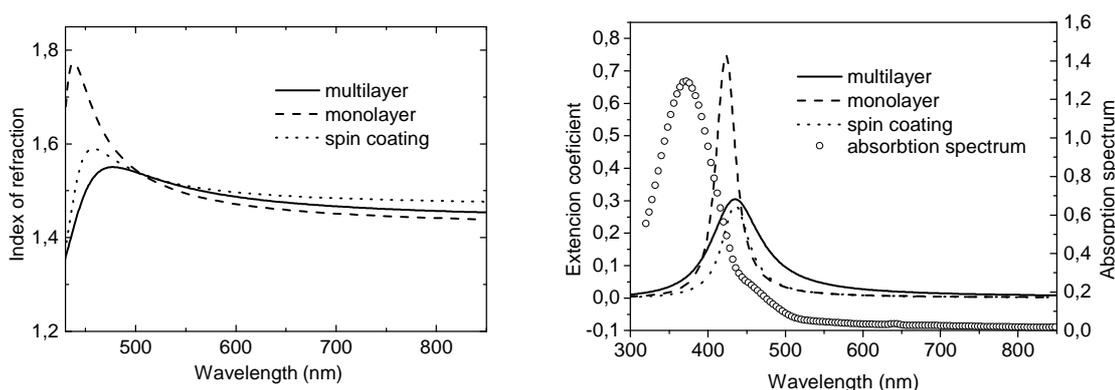
Fig. 4: *Refractive index and extinction coefficient of monolayer, multilayer film and film prepared by spin coating.*
