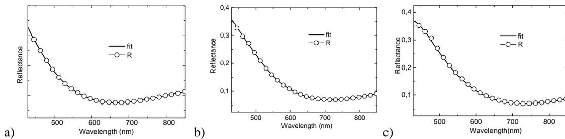
Fig. 2: Comparison of measured and fitted spectral reflectances of oligothiophene LB monolayer (a), LB multilayer (b), and spin coated layer (c).
