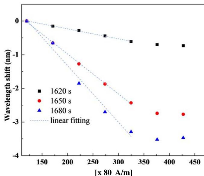
Fig. 4 Wavelength shift as a function of the magnetic field strength for SMS fiber structures corroded for different times.
