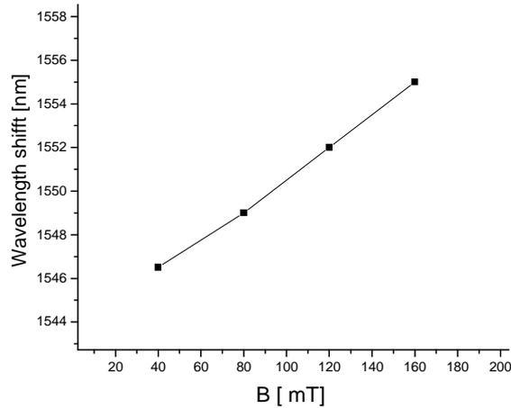
Fig. 2 The relationship between the wavelength shift and the variation of the MF strength.
