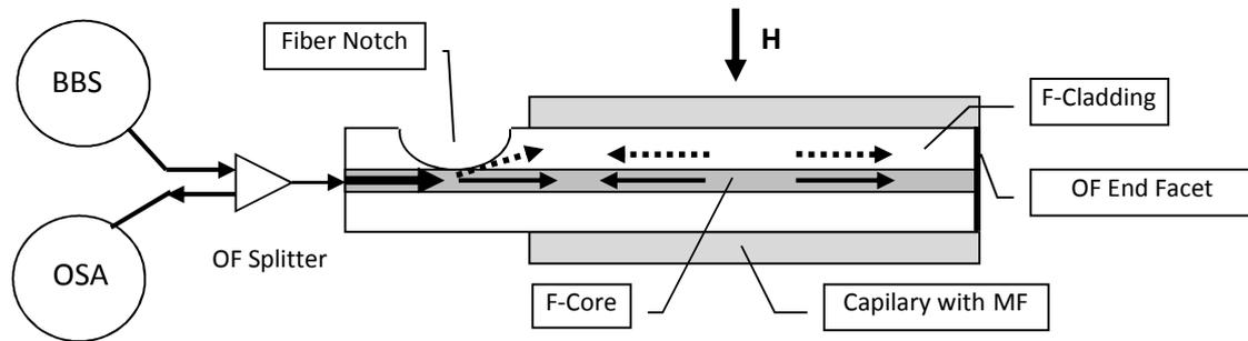
Fig. 1 Schematic diagram of the in-fiber MI based on the notch in SMF.
