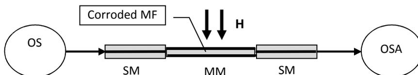
Fig. 3 The block scheme of the experimental setup for investigation of the S-M-S structure MF sensor
