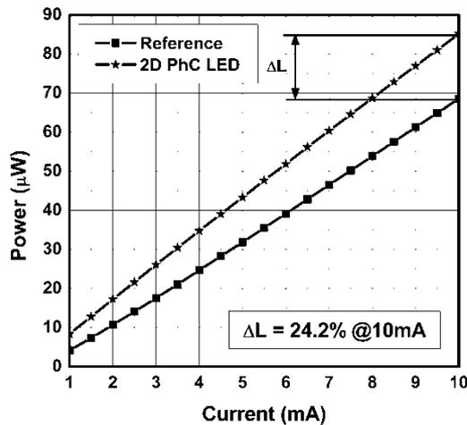
Fig. 3 Light - current characteristics measured by standard method using integrating sphere.
