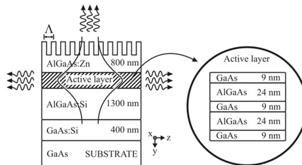
Fig. 2 AlGaAs/GaAs LED structure.
