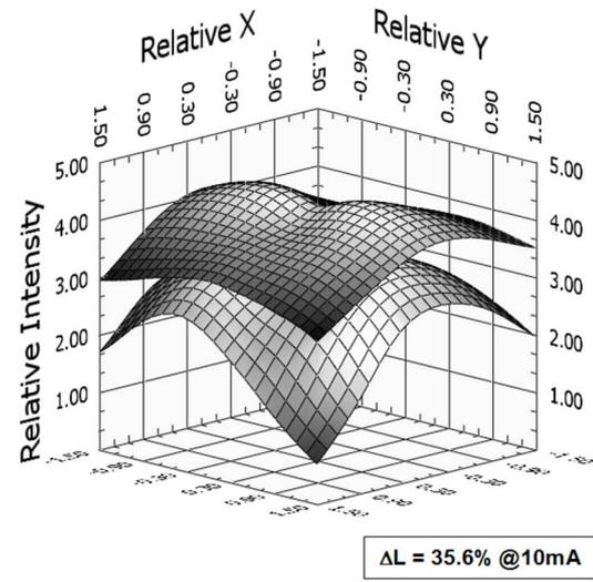
Fig. 4 Far field pattern for a) bottom: reference LED, b) top: 2D PhC LED.
