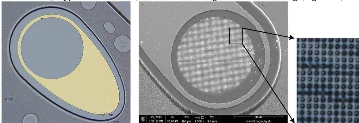
Fig. 1. SEM image of the investigated LED a) without PhC, and b) with PhC structures.
