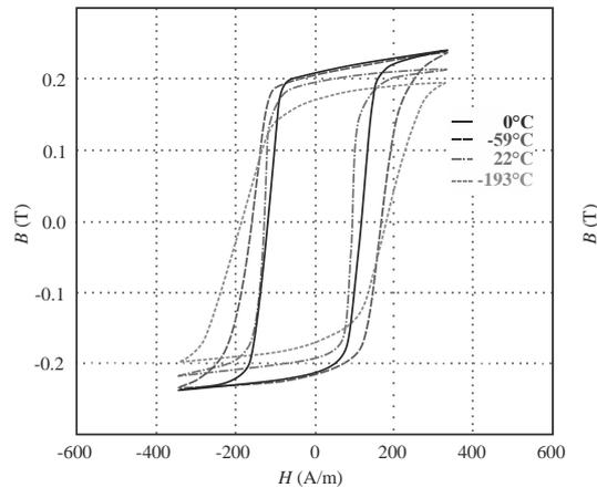
Fig. 4: *Hysteresis loops measured at applied field  $H_a = 330$  A/m for selected temperatures.*
