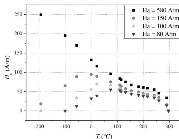
Fig. 2: The coercivity  $H_C$  as function of temperature  $T$  for applied fields  $H_a = 580, 150, 100$  and  $80$  A/m.
