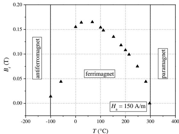
Fig. 3: Phase diagram of  $Mg_{0.347}Mn_{0.894}Fe_{1.758}O_{3.88}$  ferrite showing the three principal ground states for magnetization process at applied field  $H_a = 150$  A/m.
