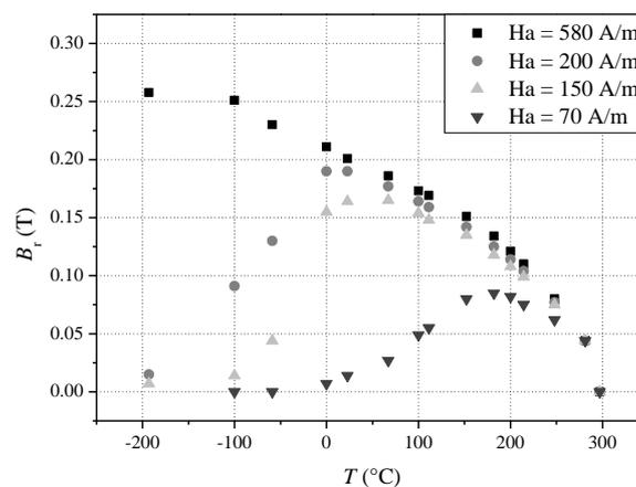
Fig. 1: The remanent magnetic flux density  $B_r$  as function of temperature  $T$  for applied fields  $H_a = 580, 200, 150$  and  $70$  A/m.
