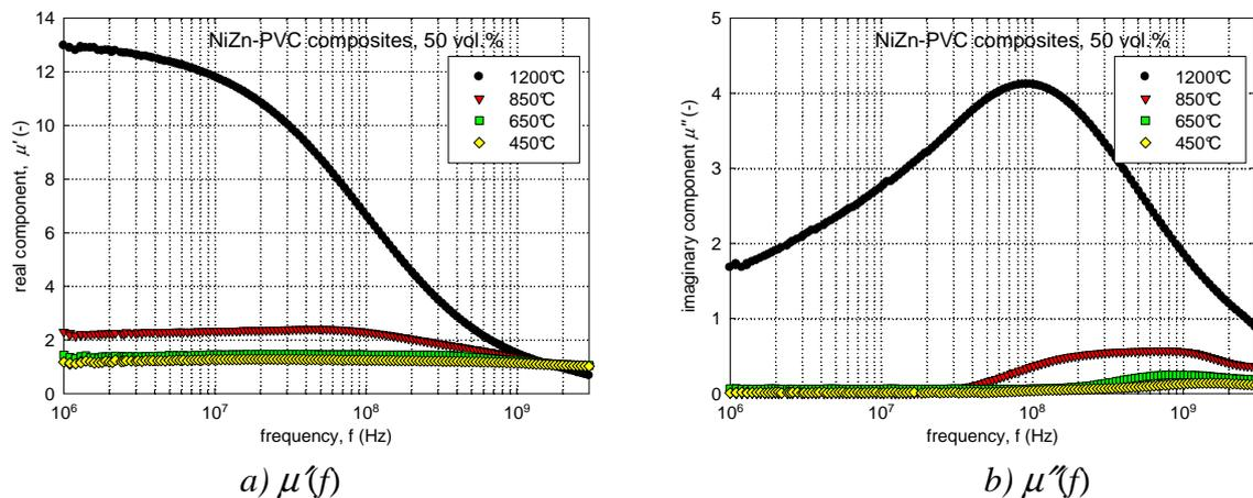
Fig. 3: Frequency dependences of real (a) and imaginary (b) parts of complex permeability  $\mu(f) = \mu'(f) - j\mu''(f)$  of NiZn-PVC composite samples.
