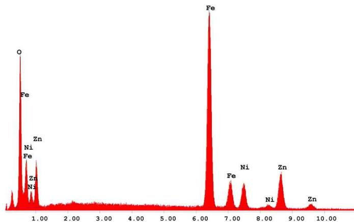
Fig. 2: EDX analysis of NiZn ferrite powder prepared at 850°C.
