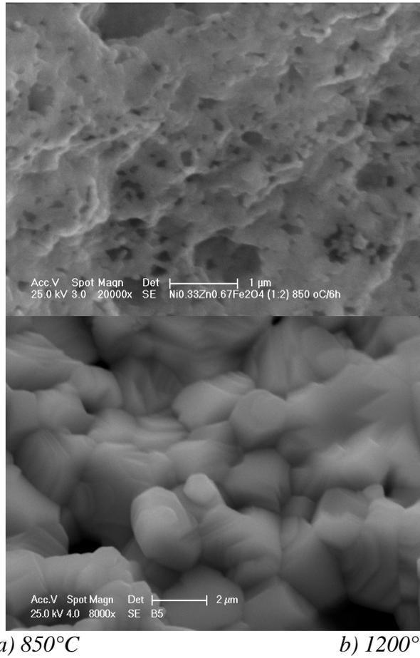
Fig. 1: SEM micrographs of NiZn ferrite powders prepared at various temperatures. Mass content of individual ions of NiZn ferrite sample calcined at 850°C is given in Table 2. The measured data fit to theoretical values of individual chemical elements very well.
