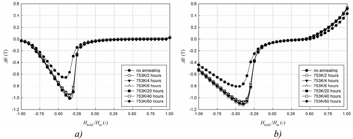
Fig.3:  $\Delta B$  as a function of  $H_{hold}/H_m$  ratio at  $f=4$  Hz, (a) and  $f=20$  Hz, (b).
