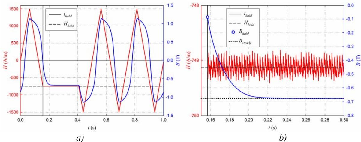
Fig.1: An example of exciting field  $H_m = 1500 \text{ A.m}^{-1}$  and corresponding flux density waveform with  $H_{hold} = -0.5H_m$ , (a) and the details of exciting field and flux density during “holding” the field, (b).
