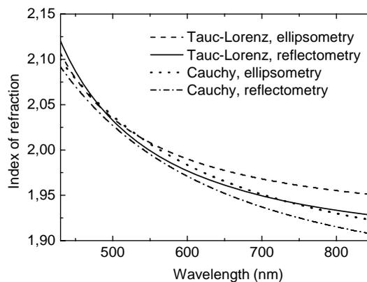
Fig. 3: Comparison of the results of ellipsometry and reflectometry. Index of refraction of the ZnO layers on glass substrate using the Tauc-Lorenz and the Cauchy model.
