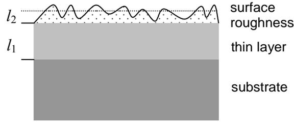
Fig. 1: Layer structure of ellipsometry model.
