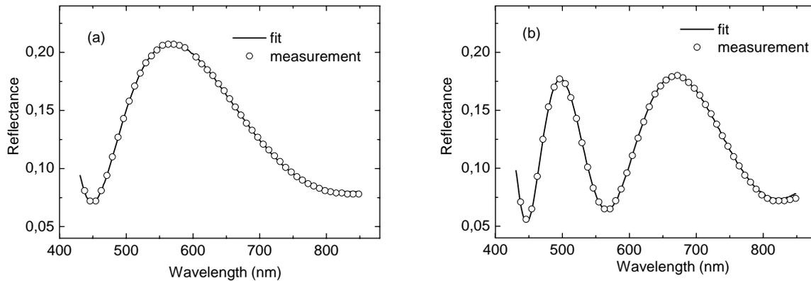
Fig. 2: Comparison of measured and fitted spectral reflectances of ZnO layers with thickness of (a) 200 nm and (b) 400 nm on glass substrate using the Tauc-Lorenz material model.
