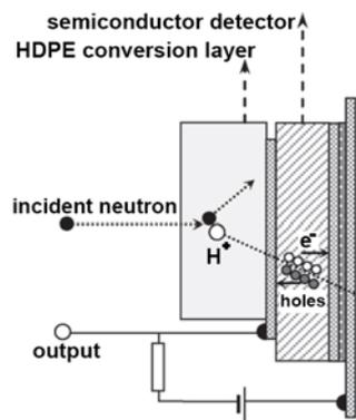
Fig. 2: *Principal scheme of a fast-neutron semiconductor detector with a conversion layer.*
