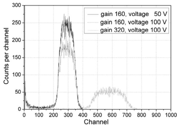
Fig. 4: Measured signal of a SiC semiconductor detector corresponding to the  $^{241}\text{Am}$ .
