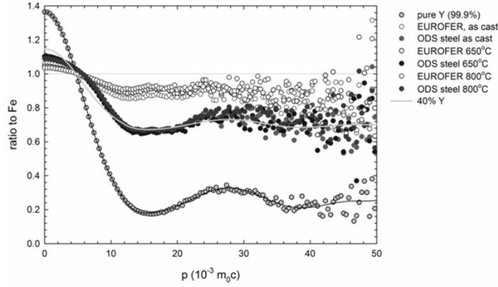
Fig. 2: CDB results of Eurofer and ODS Eurofer as cast, 650°C and 800°C and 40%, 99.9% yttrium.
