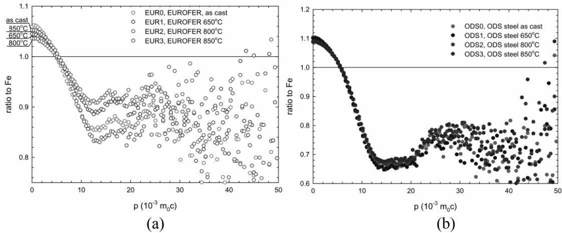
Fig.3: CDB results in detail for Eurofer (a) and ODS Eurofer (b) as cast, 650°C, 800°C and 850°C.
