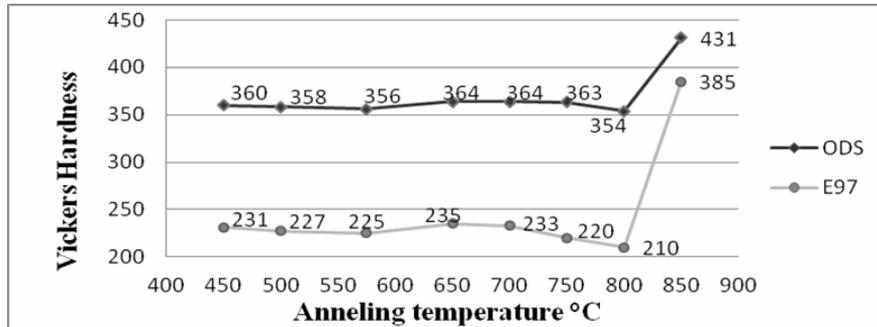
Fig. 1: HV as a function of annealing temperature for Eurofer and ODS Eurofer.
