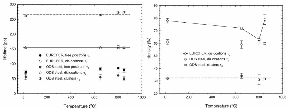
Fig. 4: Results from PALS a) lifetimes of positrons, b) intensities.
