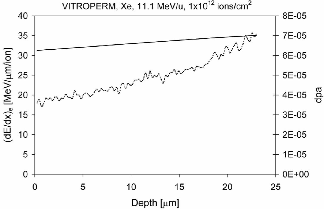
Fig. 1: Ionization (solid-line, left scale) and radiation damage (dotted-line, right scale) in VITROPERM irradiated by  $1 \times 10^{12}$  Xe ions/cm<sup>2</sup> at 11.1 MeV/u as calculated with SRIM2010. Radiation damage is expressed in dpa = displacements per atom.
