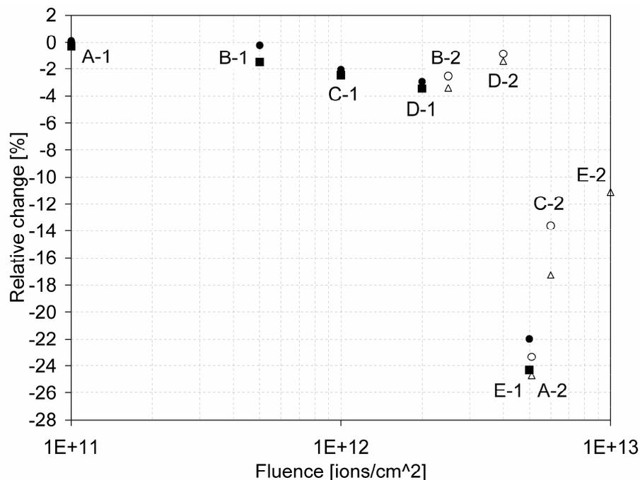
Fig.2: *Relative change of magnetic susceptibility as a function of irradiation fluence. Dark symbols=after the 1<sup>st</sup> irradiation, open symbols=after the 2<sup>nd</sup> irradiation.*
