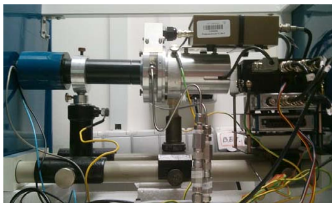
Fig.2: Mössbauer spectrometric bench for room temperature CEMS/CXMS/TMS measurements.
