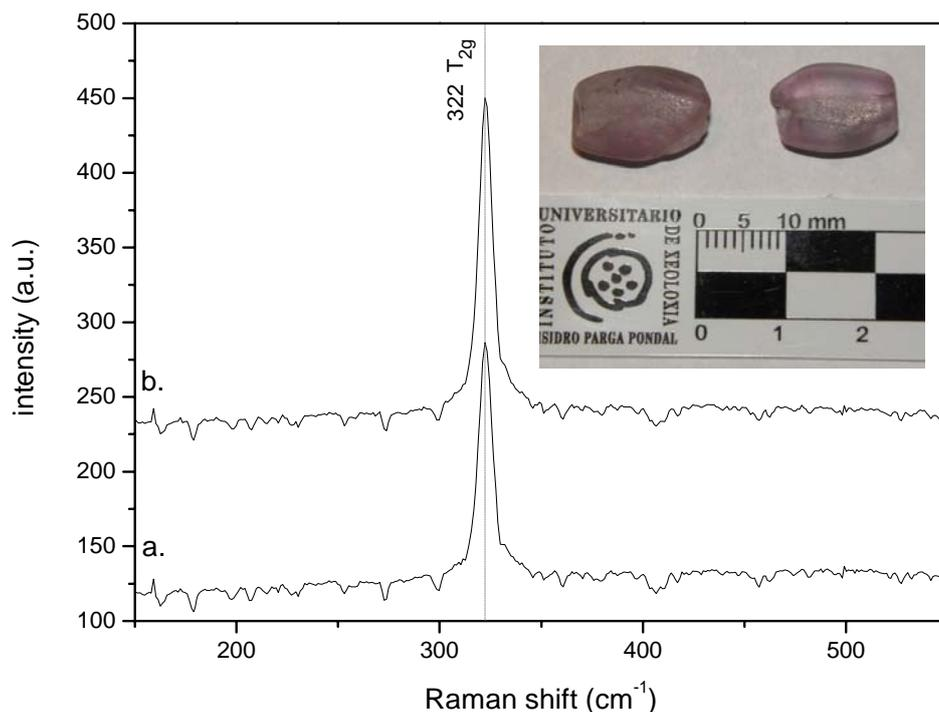
Fig. 3: Raman spectra (a) and (b) corresponding to fluorite, recorded at two different places on bead No. 3 (the left bead in the inset) of the necklace from grave 145/1985. The Raman band at  $322\text{ cm}^{-1}$  is a triple degenerated vibration of  $\text{F}^-$  anion sublattice with respect to stationary cations. This means that three vibrations have the same frequency with respect to standing  $\text{Ca}^{2+}$  cations and cannot be resolved [4].
