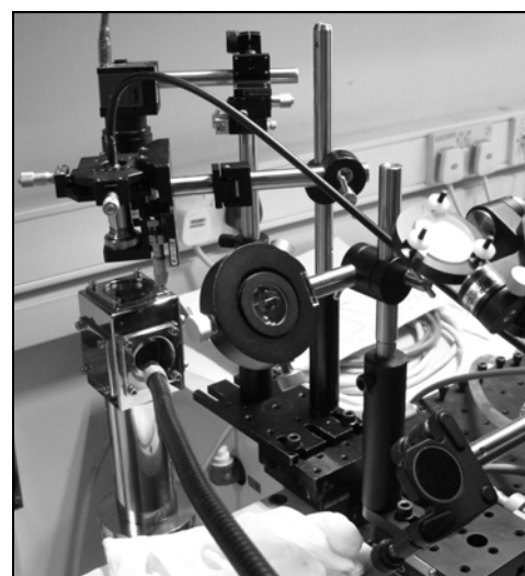
Fig.1: Sophisticated PL measurement system a) schematic b) room-temperature setup c) low temperature setup.
