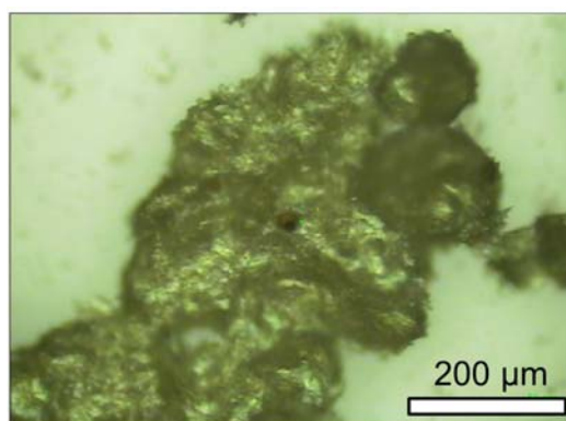
Fig.2b: Big grain on the surface of the film.
