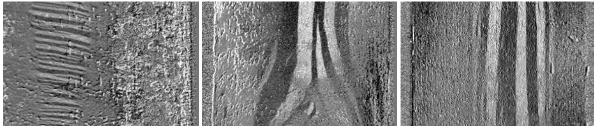
Fig.4: Domain structure of Ar annealed (no stress) Fe_{72.5}Nb_{4.5}Cu_1B_{12}Si_{10} showing: left - air side (AS), no etching; center – AS, after etching; right - wheel side (WS), after etching. (real horizontal dimension 6 mm – left and 10 mm – center and right; ribbon axis and magneto-optical sensitivity vertical besides left one where this is horizontal).
