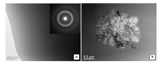
Fig. 3: *a*-Bright field TEM image and corresponding selected area electron diffraction pattern obtained from the edge of the as-cast  $Co_{47}Fe_{20.9}B_{21.2}Si_{4.6}Nb_{6.3}$  rod with 4 mm diameter, *b*-TEM micrograph of the center of  $Co_{47}Fe_{20.9}B_{21.2}Si_{4.6}Nb_{6.3}$  as-cast rod with 4 mm diameter
