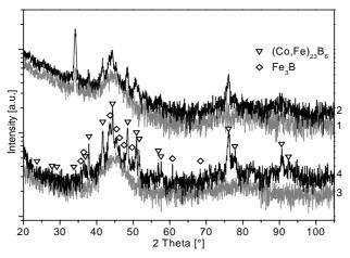
Fig. 2: XRD patterns of the as-cast Co<sub>47</sub>Fe<sub>20.9</sub>B<sub>21.2</sub>Si<sub>4.6</sub>Nb<sub>6.3</sub> samples from rods with diameter 4 and 5 mm in form of disc (curves 1 and 2) and powder (curves 3 and 4), respectively
