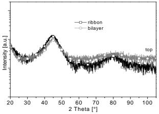
Fig. 1: XRD patterns of the as-cast ribbons and bilayer
