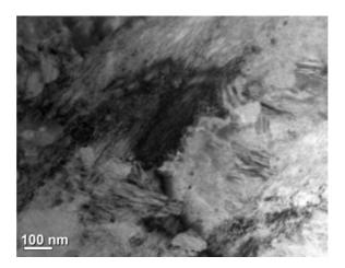
Fig. 4: TEM micrograph of the center of  $Co_{47}Fe_{20.9}B_{21.2}Si_{4.6}Nb_{6.3}$  as-cast rod with 5 mm diameter
