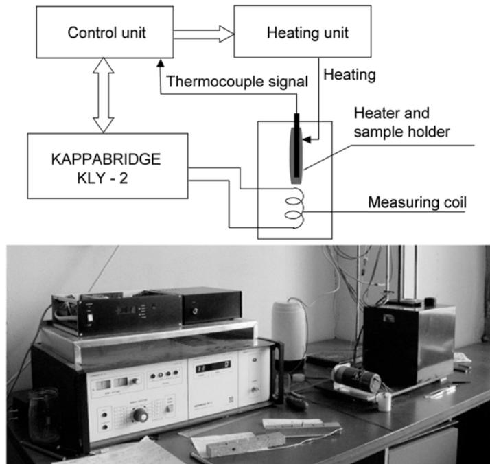
Fig.3: Kappa-bridge principal scheme (upper) and photo (lower).
