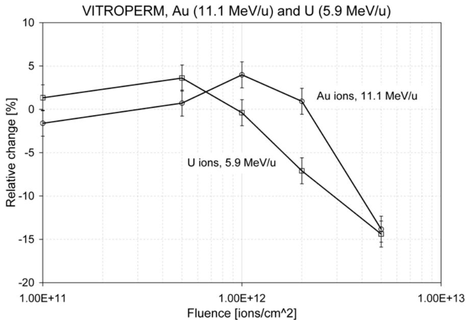
Fig.4: Relative change of magnetic susceptibility as a function of irradiation fluence, VITROPERM. Circles = Au, 11.1 MeV/u, squares = U, 5.9 MeV/u.
