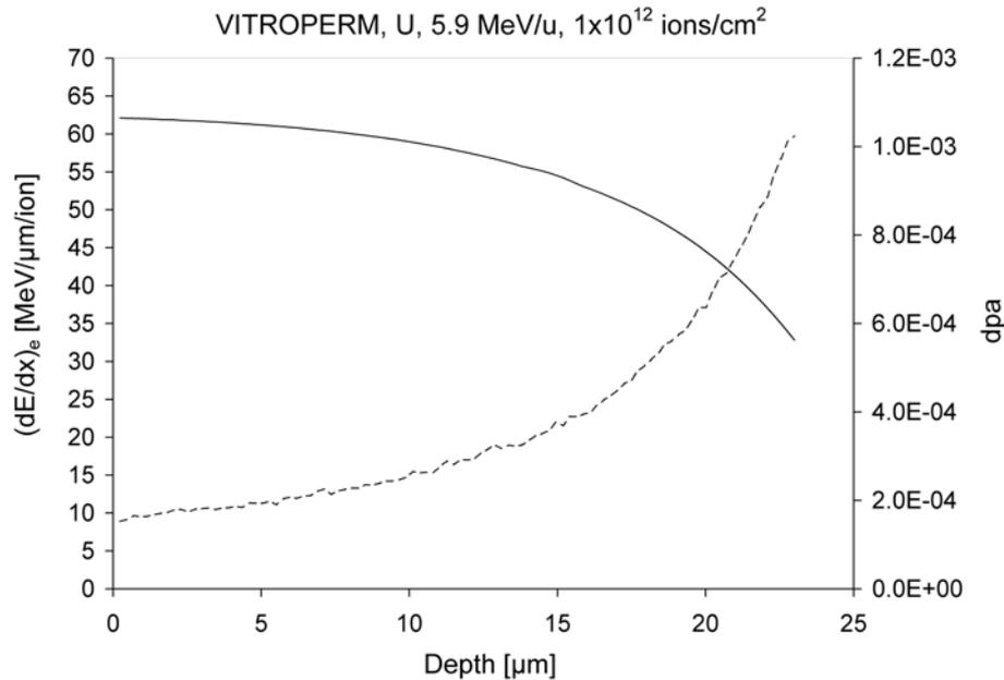
Fig.2: Ionization (solid-line, left scale) and radiation damage (dashed-line, right scale) in VITROPERM irradiated by  $1 \times 10^{12}$  U ions/cm<sup>2</sup> at 5.9 MeV/u as calculated with SRIM2010. Radiation damage is expressed in dpa = displacements per atom.
