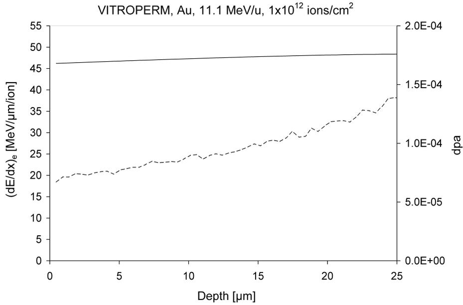
Fig.1: Ionization (solid-line, left scale) and radiation damage (dashed-line, right scale) in VITROPERM irradiated by  $1 \times 10^{12}$  Au ions/cm<sup>2</sup> at 11.1 MeV/u as calculated with SRIM2010. Radiation damage is expressed in dpa = displacements per atom.
