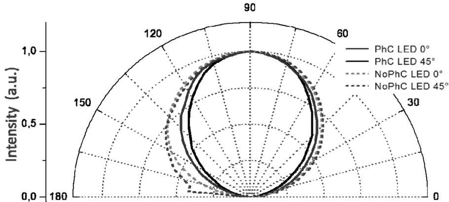
Fig. 3: a) Structure orientation for far-field radiation pattern measurements. b) Radiation pattern diagram of PhC LED and no-PhC LED shown for different structure orientations.
