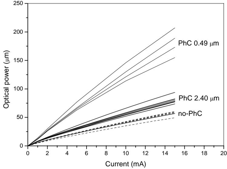
Fig. 2: Optical power vs. current for set of 2D PhC LEDs with two different periods in comparison with set of no-PhC LEDs.
