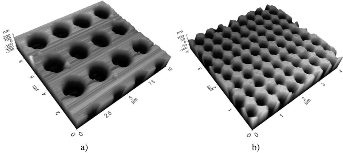
Fig. 1: AFM image of 2D PhC structures with square symmetry patterned in the LED surface with a) 2.4  $\mu\text{m}$  and b) 490 nm period.
