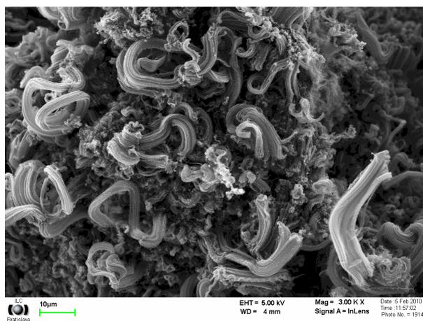
Fig. 4: SEM image of the bundles of CNT grown on Fe-montmorillonite pretreated with  $\text{Fe}(\text{NO}_3)_3 \cdot 9\text{H}_2\text{O}$ .
