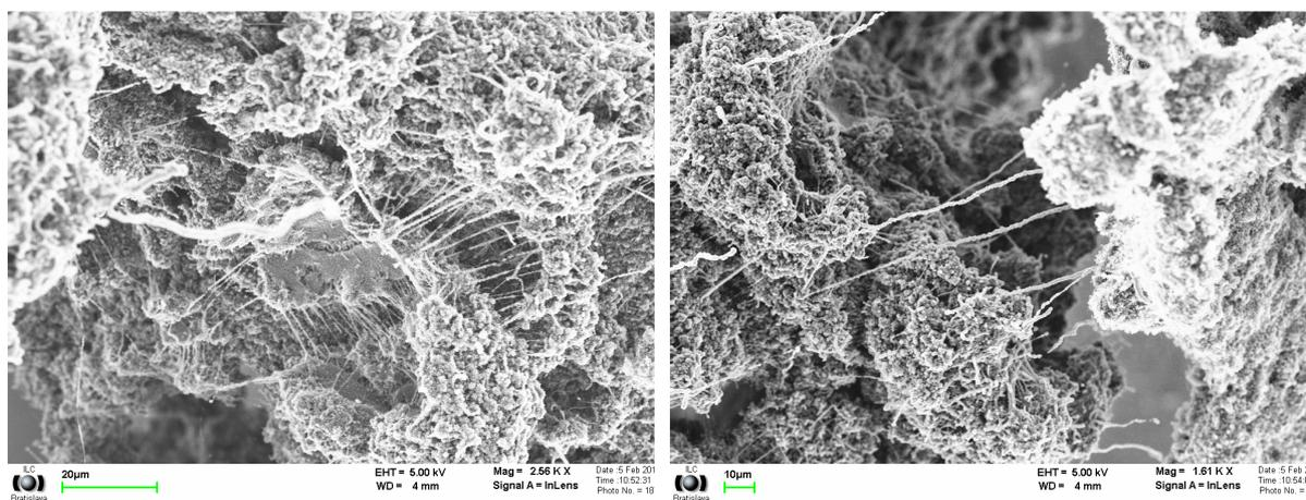
Fig. 1: SEM image of CNTs grown on Fe-zeolite pretreated with  $\text{Fe}(\text{NO}_3)_3 \cdot 9\text{H}_2\text{O}$ .
