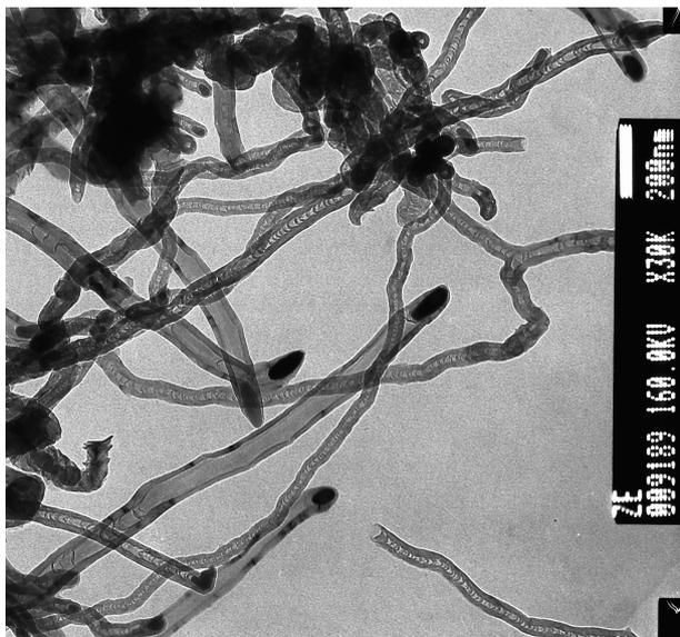
Fig. 3: TEM image of CNTs grown on Fe-zeolite. At the ends of CNTs one can see particles of the catalyst.
