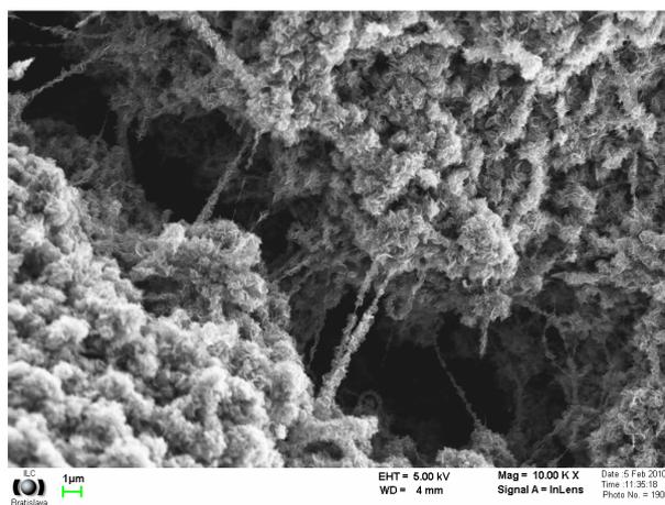
Fig. 5: SEM image of the CNT bridges grown on Fe-montmorillonite pretreated with  $\text{Fe}(\text{NO}_3)_3 \cdot 9\text{H}_2\text{O}$ . One can see the growth of amorphous carbon on CNT bridges and on the nanotubes grown in the matrix.
