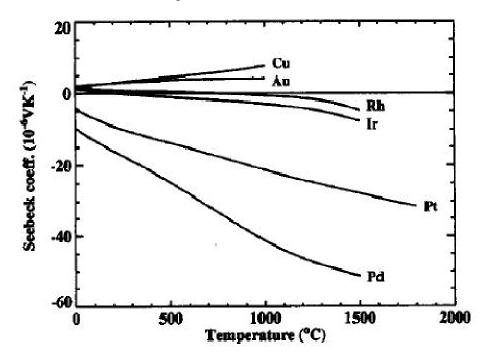
Fig. 1 - Seebeck coefficients of different elements derived from the relative rates of Pt, data EMS / and the absolute temperature coefficient for Pt.
