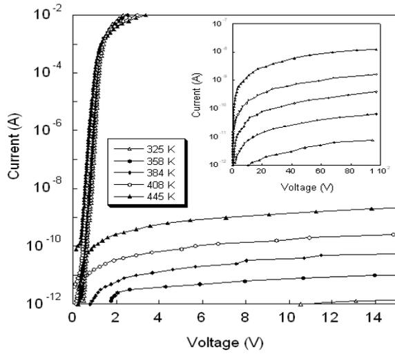
Fig. 2: *I-V* characteristics of a typical Au-Ni/4H-SiC Schottky barrier measured at different temperatures. The ideality factors of the diodes, calculated in the current interval of  $10^{-9} \div 10^{-5}$  A, are in the range of  $1.2 \div 1.4$ . The reverse characteristics up to 100 V are shown in the inset.
