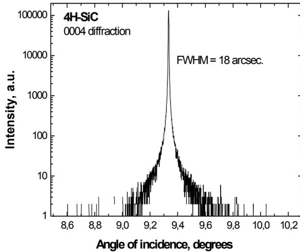
Fig. 1: High resolution X-ray diffraction of the 4H SiC epitaxial layer. The optimum crystal order is confirmed by the FWHM of the peak.
