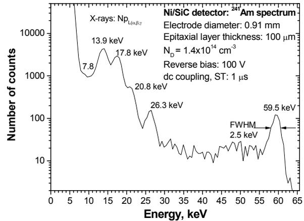
Fig. 5: Pulse-height spectrum of the  $^{241}\text{Am}$  radionuclide revealed by the fabricated 4H-SiC detector plotted in semi-log scale.
