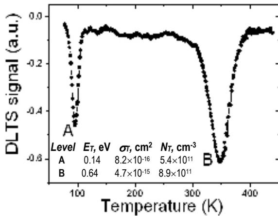
Fig. 4: DLTS spectrum of the Au-Ni/4H SiC Schottky barrier: pulse frequency 264 Hz, pulse width 135  $\mu\text{s}$ , reverse voltage -3 V, pulse voltage 0 V.
